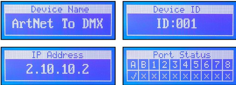
There are 4 initial “top-tier” menu status screens (shown above) that you’ll see when you power on the unit. You can scroll through them by using the **<UP/DOWN>** buttons. The **Device Name**, **Device ID**, and **IP Address** can all be edited later within the menu settings.
