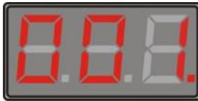
The decimal point of last digital of the display tube will twinkle regularly when receives DMX512 signal normally.
